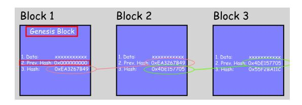
$\rightarrow$  chain (via hashing) of blocks (data, "txs", "state")
